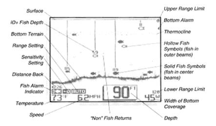
The 2D view provides more information about bottom hardness and texture using Structure ID. Only information collected from the center two beams is used to draw the bottom depiction. Terrain outside the coverage area of the center two beams will not be seen in the 2D view. Using a narrower beam provides much more detailed information as to the composition of the bottom.
